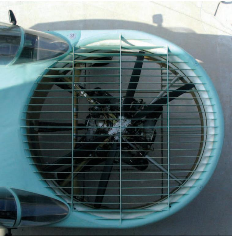
notably, the X-Hawk's lack of an exposed rotor will make it much more flexible than present-day helicopters, allowing it to enter more confined areas safely or even make physical contact with buildings while hovering if necessary.
