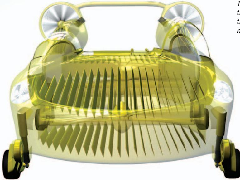
This computer-generated cutaway image of the X-Hawk illustrates the internal layout of the tandem ducts with their patented multiple-vane control system.
