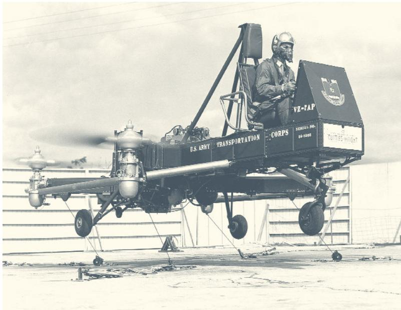
*The Curtiss-Wright VZ-7AP, shown during tethered flight tests with the ring guards removed.*
