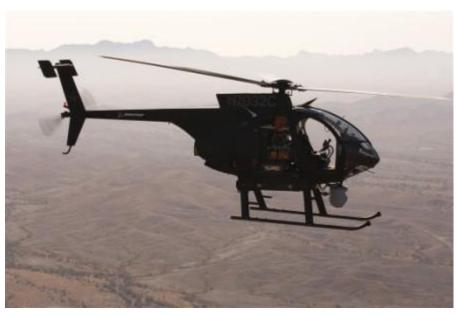
Boeing Mesa flew its Unmanned Little Bird (ULB) demonstrator for the first time without a safety pilot June 30 at the U.S. Army's Yuma **Proving** Grounds in Arizona. The modified MD 530F helicopter lifted off from a helipad, hovered briefly, and flew a programmed 20minute armed intelligence,
