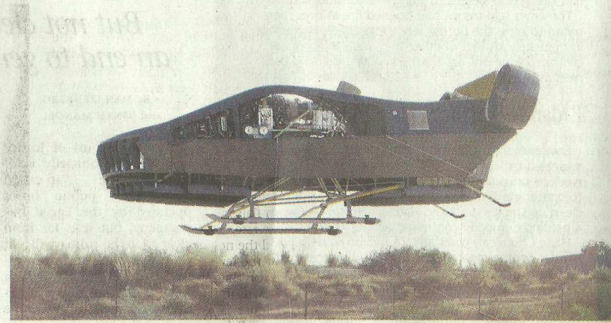
GETTING SOLDIERS to safety. The AirMule unmanned aerial vehicle can fly like a helicopter and evacuate the wounded from anywhere.
