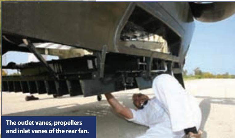
The outlet vanes, propellers and inlet vanes of the rear fan.
