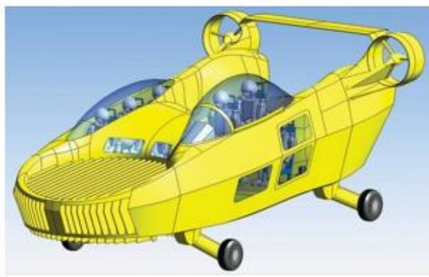
The Israeli-designed X-Hawk would use directed fans to take off vertically and fly up to 155 mph.
