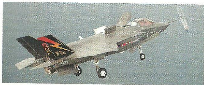
Shaft-driven lift fan activated from a forward air speed of 180kt
